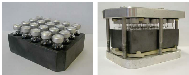
Figure 2. High-throughput synthesis platform for parallel microwave chemistry in silicon carbide plates. The left image shows the experimental setup for low pressure applications utilizing HPLC/GC vials with aluminum crimp tops for reaction temperatures of ~250 °C (max pressure ~8 bar). The right image shows the high pressure setup utilizing an aluminum sealing plate for achieving the reaction temperatures of 250 °C (max pressure 20 bar) used in this work. For further details, see ref 15.
